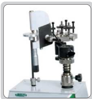
check the measuring force of indicating micrometers
