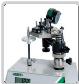
check the measuring force of bore gauges
