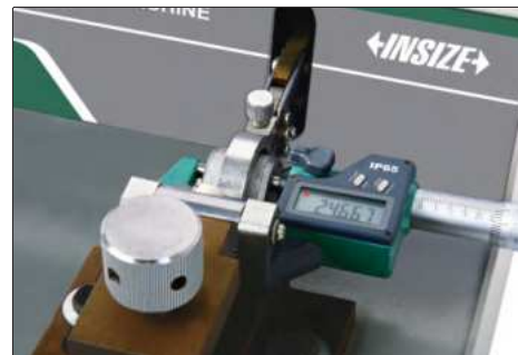
lapping measuring surfaces of outside micrometer
